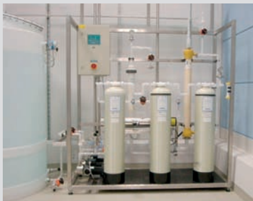
Processing plant for highly purified water/clean room applications / Reinstwasser-Prozessanlage/Reinraumapplikation
