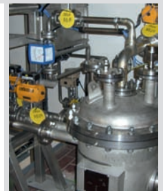
Cake building filtration/ Kuchenbildende Filtration
