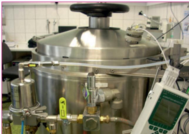
Fig. 1: Waste air filter system of a laboratory autoclave with the measurement path of an adapted water intrusion test
