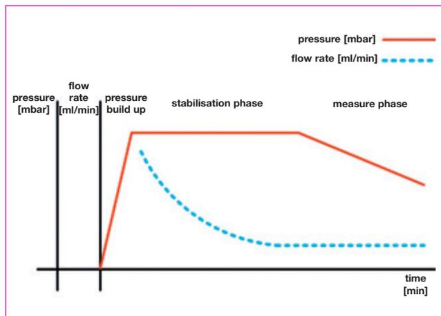
Fig. 2: Pressure drop method (schematically)
