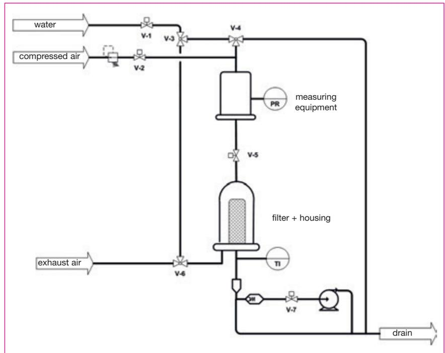
Fig. 3: Flow chart of the measurement system adapted to the waste air filter system of an autoclave
