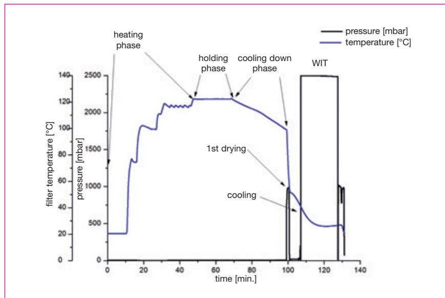
Fig. 6: Sterilisation procedure
