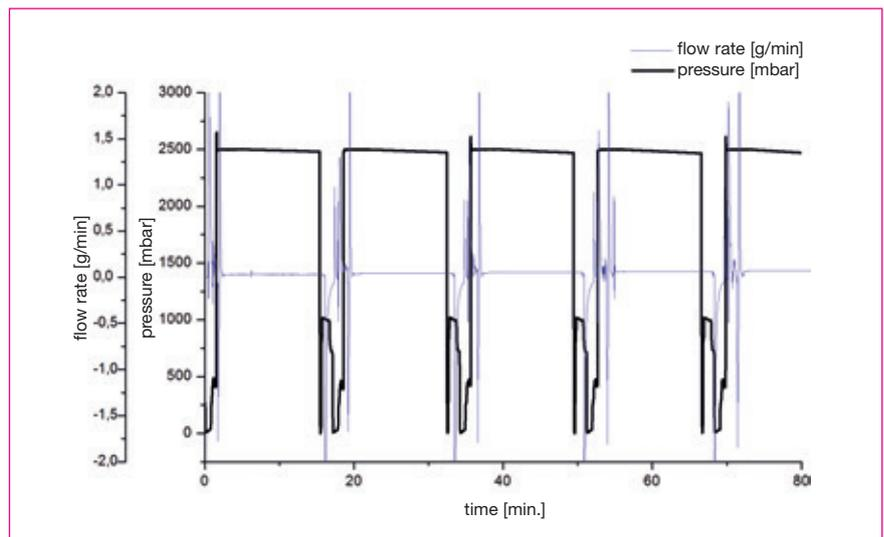
Fig. 4: Automated calibration sequence of the test system
