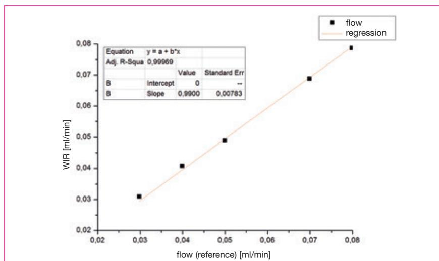
Fig. 5: Calibration curve (flow calibration)
