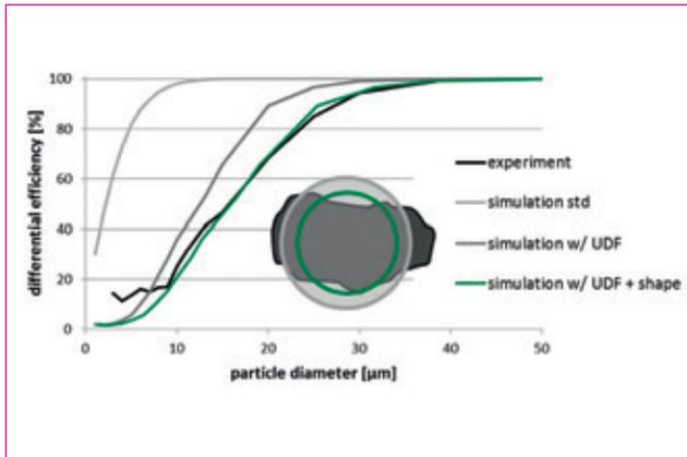
Fig. 6: Comparison of different separation efficiency calculations with measured data
