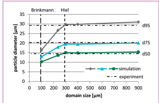
Fig. 7: Comparing measured data with simulation results for particle sizes, with the separation efficiency set in accordance with the domain size
