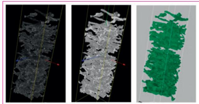
Fig. 2: Example of a 3D fiber structure (from left to right) Raw data from the XCT image, segmented fiber structure in MAVI, fibers imported as voxels in GeoDict.
