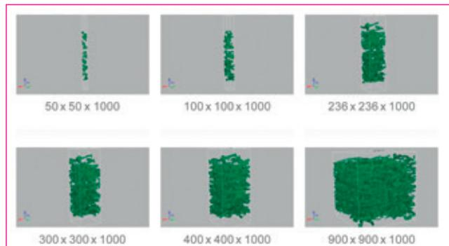
Fig. 4: Fiber structure image for different domain sizes (Resolution: 1 voxel = 1 μm)
