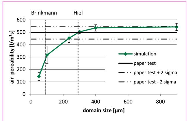
Fig. 5 – Initial pressure drop – simulations for various domain sizes compared to the target range of twice the standard deviation from the measurement results (DIN EN ISO 9237) (♦♦ new formula)
