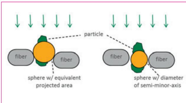
Fig. 3: How the choice of characteristic diameter determines filtration
