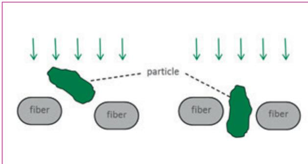
Fig. 1: Diagram showing the passage of non-spherical particles through a fiber structure
